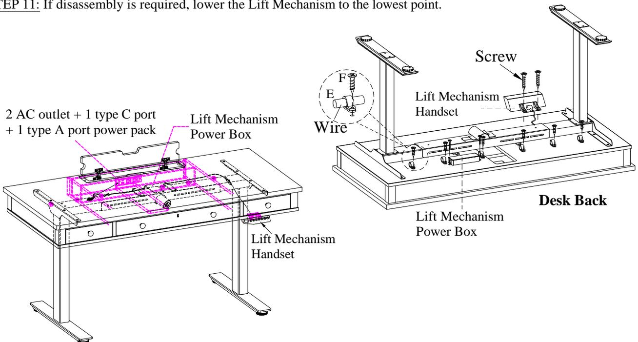
Note: Refer to Lift Mechanism assembly instructions for Handset operation.
