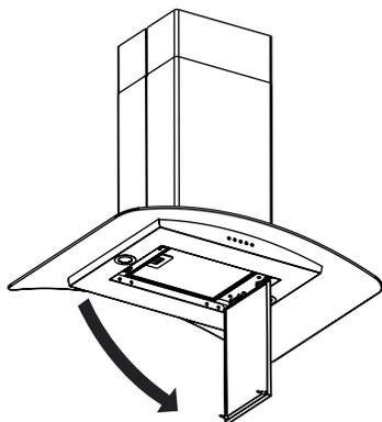
2. Remove the filter by pulling the spring release handle and then pulling down the filter.
