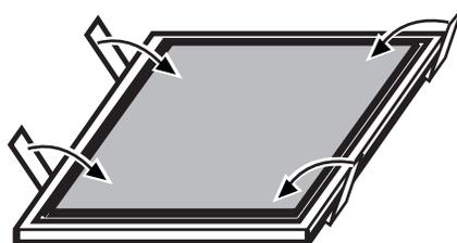
5. Replace metal grease filter. See “Metal Grease Filter” in this section.
