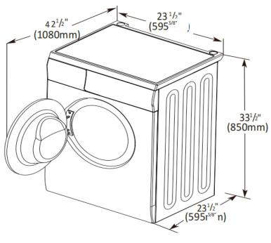
The dimensions shown are for the recommended spacing. Custom undercounter installation.
