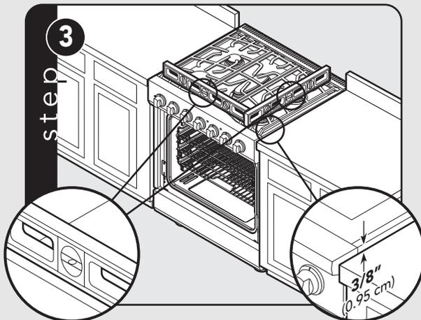
Check that unit is level side to side and front to back. The side trim must be 3/8" (0.95 cm) above countertop. If unit is not level, repeat Steps 5-7 in "Leveling/Adjustments/Alignment" section.
