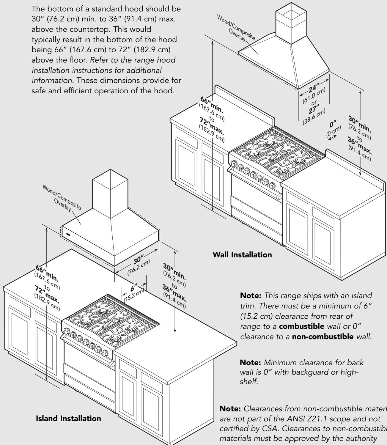
**Note:** This range ships with an island trim. There must be a minimum of 6" (15.2 cm) clearance from rear of range to a **combustible** wall or 0" clearance to a **non-combustible** wall.
