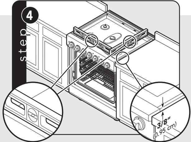
Check that unit is level side to side and front to back. Side trim of the high corner must be  $\frac{3}{8}$ " (0.95 cm) above countertop.
