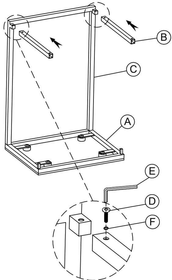
Step 3: Using the Allen key to tighten all bolts.
