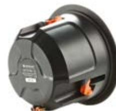
Regardless of interior ceiling or wall construction, the Controlled Performance range guarantees sonic consistency. We fit all models with fully-sealed back boxes, providing an ideal air load for the drivers and optimising audio performance. These rigid, mineral filled enclosures reduce the sound from the back of the cabinet by around 15 to 22 dB. This range guarantees excellent audio quality and versatility, for superior levels of sound isolation between rooms and floors.
