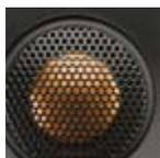
**C-CAM Gold Dome Tweeter:** The Gold Dome tweeter is formed from a Ceramic-Coated Aluminium Magnesium alloy, Gold anodised to a specific thickness for ideal stiffness and damping characteristics. Thinner, lighter, more rigid and more efficient than domes made from other materials which are prone to distortion in the audio band.
