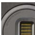
**MPD High Frequency Transducer:** Micro Pleated Diaphragm high frequency transducer uses a proprietary low-mass pleated diaphragm with a surface area eight times larger than that of a traditional dome tweeter. MPD transducers work like a super-fast accordion by rapidly squeezing the pleats to produce a smooth, wide, naturally fast response up to 100 kHz.
