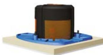
The CFB3-KIT retrofit installation kit cleverly provides a firm fixing behind plasterboard/Sheetrock and requires just three bolts to complete the fit. **NOTE:** The retrofit option is not flush fitting, but requires no plastering. The grille will sit slightly proud of the ceiling surface by 3.55 mm, less than a standard In-Ceiling grille.
