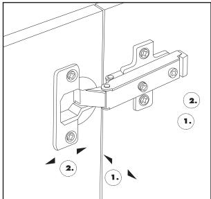
Use the **Phillips Screwdriver (A)** supplied to adjust Vertica's door hinges:
