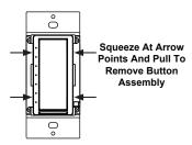
**NOTE**: When the button assembly is removed, power to the unit and load is removed automatically
