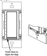
**NOTE**: Power is automatically disconnected when the button assembly is removed. For instructions on removing the button assembly, refer to "Changing Button Assemblies" on the previous page.
