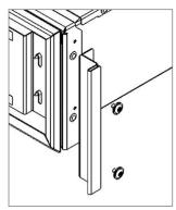
2 For black glass and stainless steel front panels, proceed to step 5. For custom drawer fronts, remove the four screws from the back of the front panel assembly.
