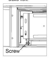
7 Align the drawer front tabs with the openings on the drawer front and the lower mounting brackets with the mounting screws.
