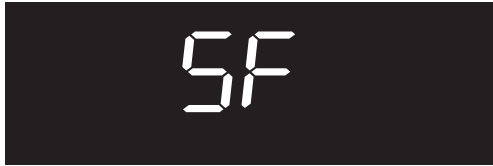
Figure 28: Display showing Sabbath failure
