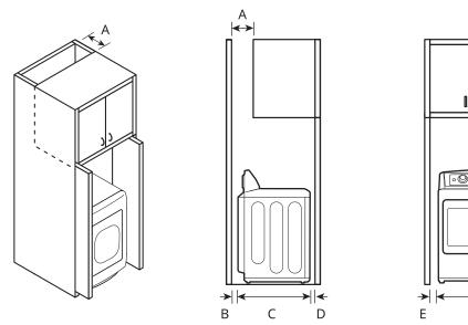
For cabinet installation with a door, minimum ventilation openings in the top of the cabinet are required.
