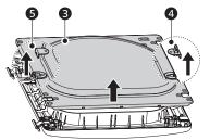
Remove the 4 screws is securing the hinges to the door frame. Remove the two plastic cover caps in the new security. Reinstall the hinges is and cover caps in the opposite sides from which they were removed.
