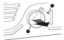
2 Press the adapter duct ③ onto the blower housing and secure it to the base of the dryer as shown.
