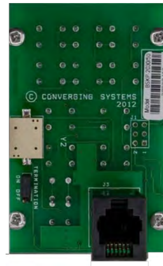
Figure 20. Rear of wall switch with RJ25 input
