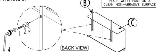
STEP 2 : Assemble the Mirror Support (B) with the Mirror (A) by using Allen Key (4) with hardware 1, 2 and 3.
