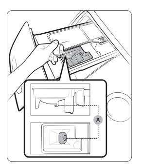
**3.** Add fabric softener to the **softener compartment**. Do not exceed the **max line (A)**.
