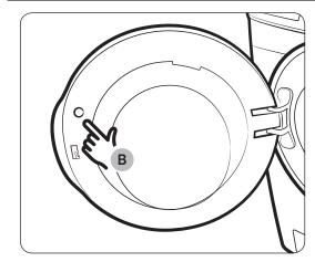
Remove the **small circle film (B)** above the door latch before use.
