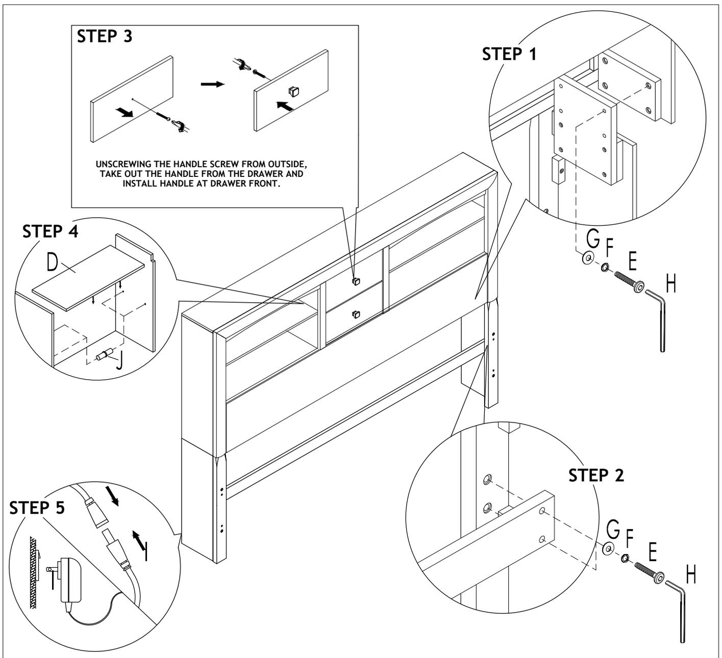
NOTE : MUST TIGHTEN SCREWS PERIODICALLY. WITH USE SCREW MAY BECOME LOOSE. CHECK TIGHTNESS OF ALL SCREWS EVERY 6-8 WEEKS.
