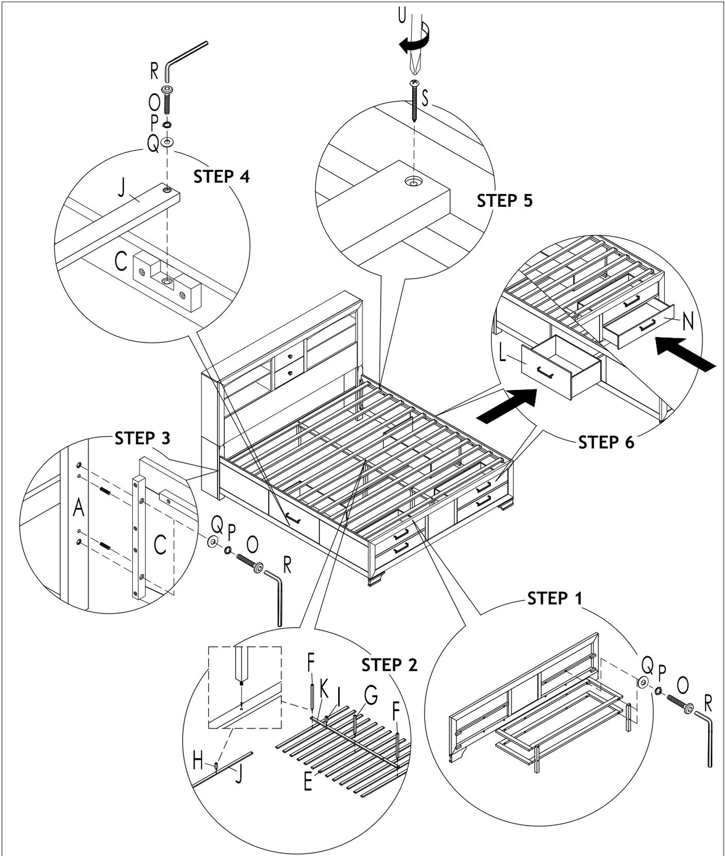
NOTE : MUST TIGHTEN SCREWS PERIODICALLY. WITH USE SCREW MAY BECOME LOOSE. CHECK TIGHTNESS OF ALL SCREWS EVERY 6-8 WEEKS.
