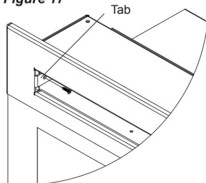
3. Use the supplied two Phillips sheet metal screws to fasten the glass assembly tabs to the fireplace (Figure 17).
