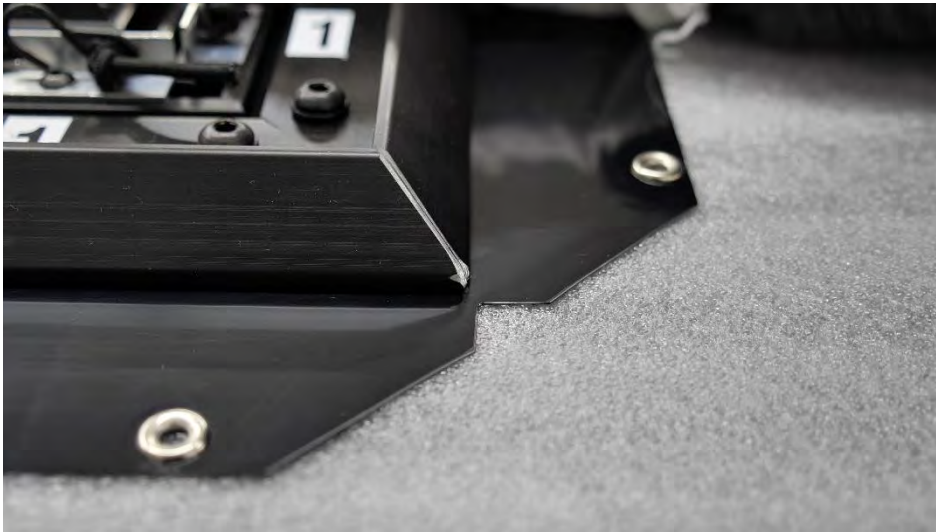
Figure 17: Align corners of screen with corners of frame
