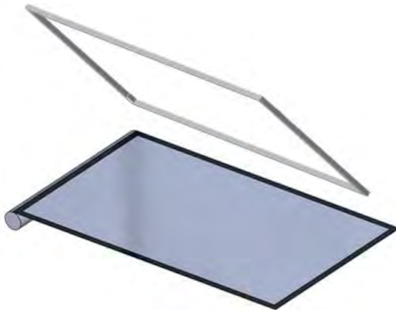
Figure 15: Unrolling the screen material, viewing side down
