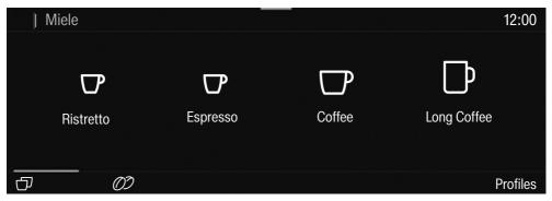
The menu path appears on the left of the **header**. If you touch a menu name in the header, the display will switch to that menu. To switch to the start screen, tap  $\triangle$ .
