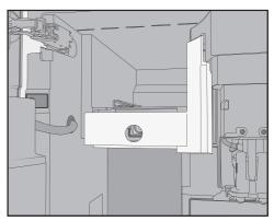
Remove the milk valve cover: press on the recessed grip to unlock the cover.
