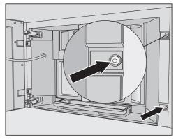
2 screw holes are fitted with red silicone plugs to protect the appliance against transport damage and secure the door during transport.
