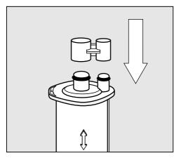
**Useful tip:** You can seal the descaling cartridge with the cap that can be found on the cartridge. This cap can be easily detached by snapping it off.
