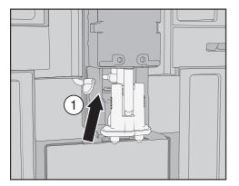
■ Detach the milk pipework from the dispensing unit as follows: pull the tab (1) to the left.
