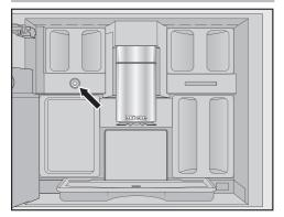
The milk valve is located under the bean container on the left-hand side.
