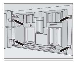
Four TX20 (25 mm) screws are supplied with the machine.
