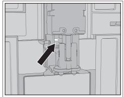
Do not remove the milk pipework connecting piece. If necessary, clean the connecting piece with the cleaning brush.
