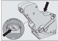
■ Wipe any coffee grounds from the filters. One filter is located in the funnel and the other to the left of the funnel.
