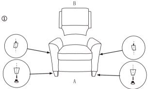
1. Please assemble the legs first before turning over the chair in order to avoid motor broken. Take down the bag from the bottom of the chair, legs are packed inside. Assemble the legs as the picture shows above.
