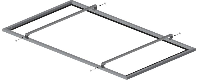
Figure 6: Temporarily Attaching Wall boards to the Frame
