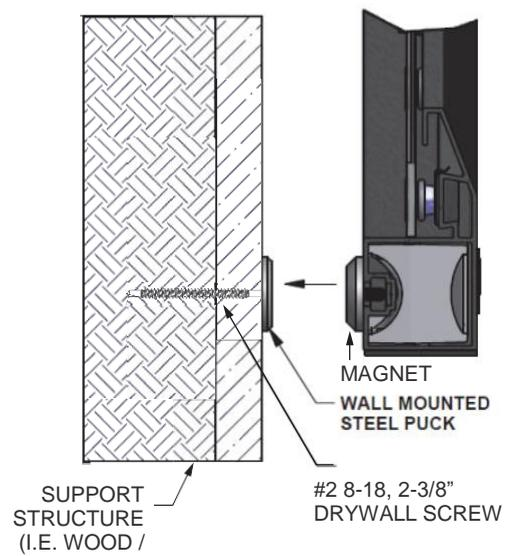
Figure 5: Wall Mounting - Side/Bottom View
