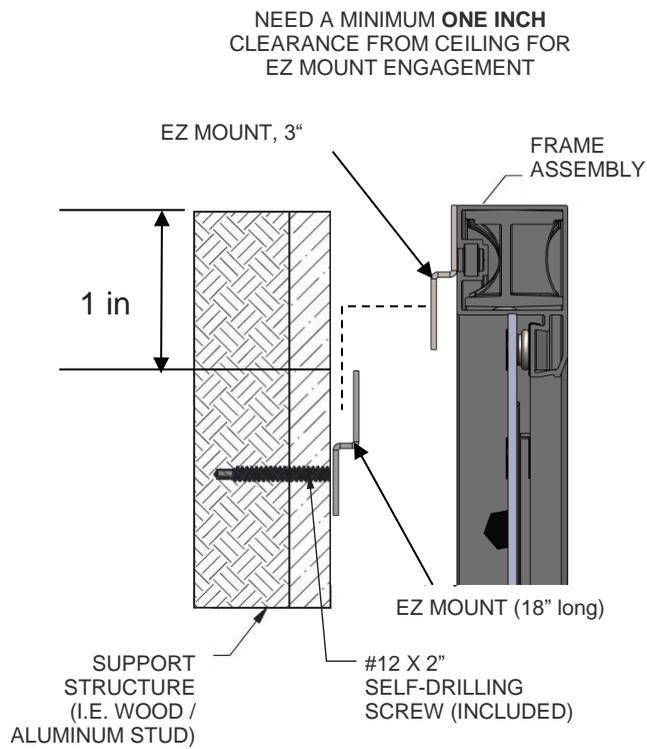
Figure 4: Wall Mounting - Side/Top View
