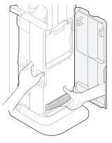
**5** Remove dust from the motor protection filter and exhaust filter once every 3 months and wash them using room temperature water.
