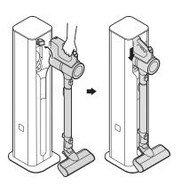
2 When the dust emptying operation is complete, a melody sounds, the dust emptying (replace bag) icon turns off, and the vacuum cleaner starts charging.
