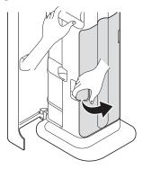
**3** Press ▲ button **①** above the **PUSH** label with one hand. The dust bag is released.
