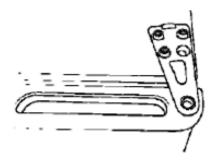
2. Unscrew the three screws from the metal bracket, and set aside. Carefully remove the door, and place it on a cushioned surface.
