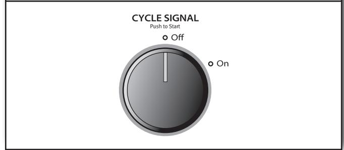
Turn the Cycle Signal knob to select the desired setting (On or Off). The Cycle Signal produces an audible sound when the drying cycle is finished. Promptly removing clothes at the end of the cycle reduces wrinkling.
