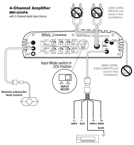
To LEFT and RIGHT Speaker Terminals of head unit or signal processor
