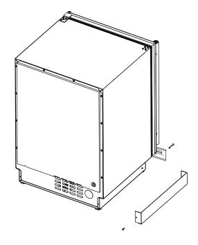
3. Align front hole wit hole in shell accessory, hole in base, and hole in grille. Tighten screw.
