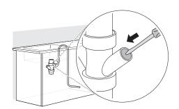
Attach the drain hose to the waste tee with the hose clamp provided. Move the clamp into position and tighten it with a flat-blade screwdriver.
