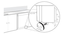
3 Use a Phillips screwdriver to remove 2 screws
