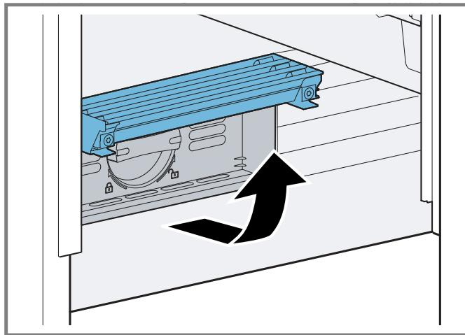
2. Turn the water filter counterclockwise by 90° ① and remove it ②.
