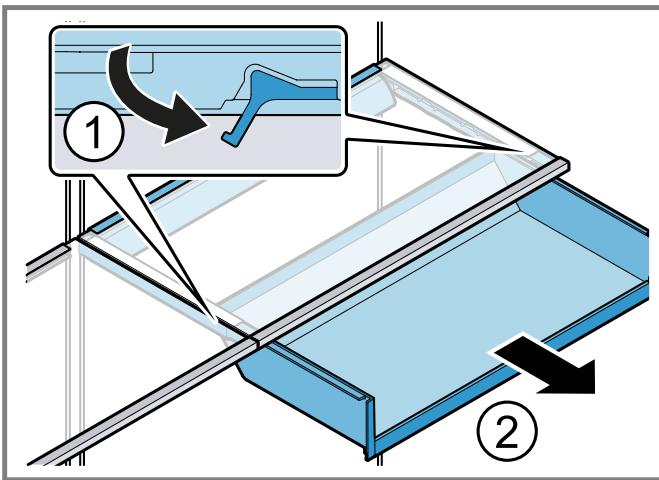
2. Underneath the cool-fresh container on both sides, press the telescopic rail lock outwards ① and remove the cool-fresh container ②.
