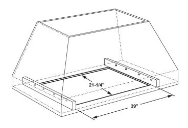
These hoods are secured to the custom cabinet from both sides through 8 screws.
