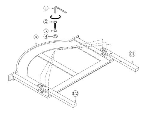
STEP 2 Assemble the headboard cross bar (D) to headboard legs (C1 & C2) by using Allen Key (1) with hardware 2, 3, and 4. \*TIGHTEN ALL THE BOLTS BY USING ALLEN KEY (1)
