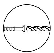
2. Match the drill bit to the wall anchor and hole size.
