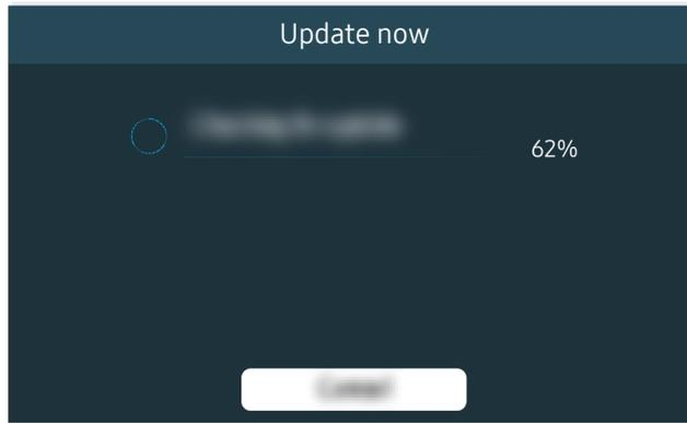
The firmware update begins automatically. Your TV will automatically powercycle when the firmware update is completed. Do not turn off your TV while the firmware update is in progress.
