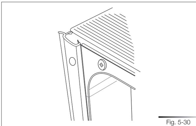
Tighten the supplied screws with a screwdriver; this operation definitively fixes the dishwasher to the adjacent units; cover the side holes using the supplied plugs (ref. A fig. 5-31).
