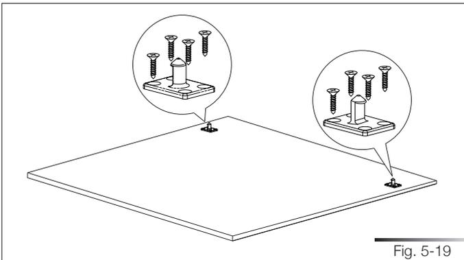
Drill holes for the panel handle using a drill with a suitable bit. Use the screwdriver to secure the door handle before hooking the panel to the dishwasher (see fig. 5-20).
