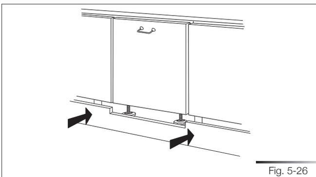
Before securing the dishwasher to the adjacent units, attach the gaskets to the sides.
