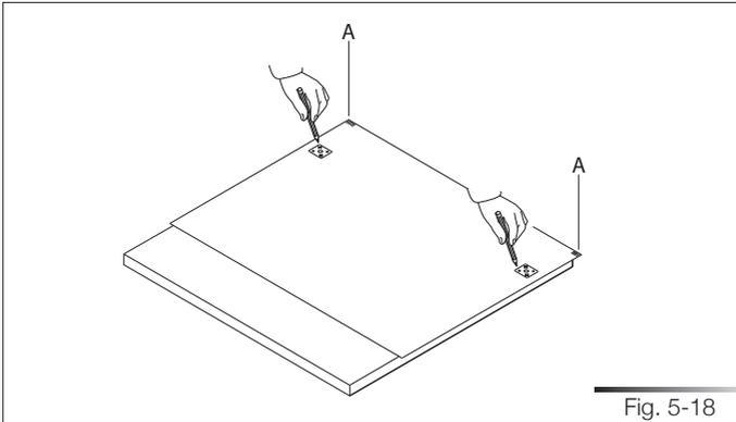
Use the screwdriver to secure the door hooks with the 8 supplied screws (see fig. 5-19) at the marked reference points.
