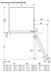
The drawing is based on a cabinet panel width of  $^3/4^\circ$  (19 mm) and a Gaggenau cabinet handle height of  $1^5/16^\circ$  (49 mm).
