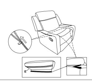
Step 4: Pull out handle to open the footrest as shown below diagram .
