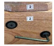
3. After attaching all legs make sure they are fixed firmly and not shaking.
