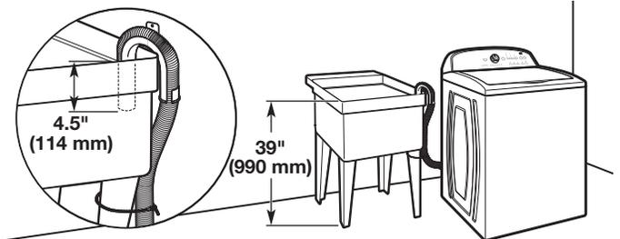
Minimum capacity: 20 gal. (76 L). Top of laundry tub must be at least 39" (990 mm) above floor; install no higher than 96" (2.44 m) from bottom of washer.
