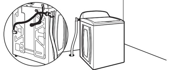
Floor drain system requires a Siphon Break Kit (Part Number 285834), 2 Connector Kits (Part Number 285835), and an Extension Drain Hose (Part Number 285863) that may be purchased separately. To order, please see toll-free phone numbers in your Use and Care Guide. Minimum siphon break: 28" (710 mm) from bottom of washer. (Additional hoses may be needed.)
