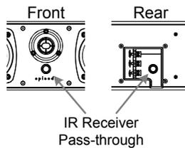
To maintain accurate IR reception, a spacer has been included to allow for the front edge of the IR receiver to be flush with the back of the grille cloth. This will ensure that IR reception is at its maximum level.
