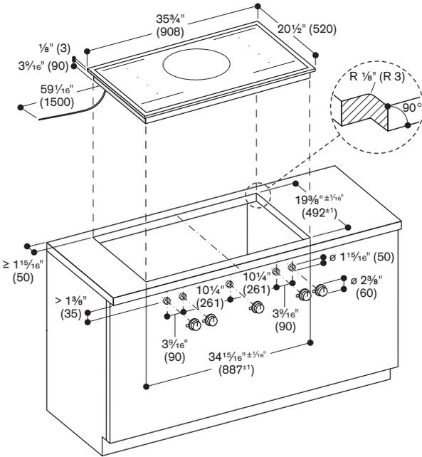
Minimum countertop thickness  $\frac{3}{4}$ " (20 mm) for surface mounted installation. See separate planning notes on page 104.
