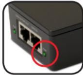
**Reset Button:** The Reset button is located on the bottom panel of the XAP-1240 and is used to restore factory default settings. To Restore Default Settings, with the XAP-1240 powered on, press and hold the Reset button for 10 seconds, then release.
