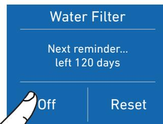
Here are indicated the remaining days before replacement of the filter.
