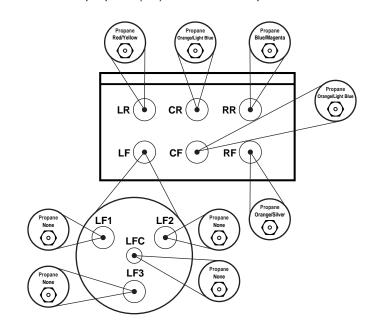
To prevent leakage, make sure the orifice spuds are securely screwed into the gas supply tubes.
