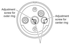
Adjustment screws for multi-ring burner only
