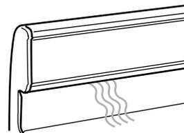
The oven vent releases hot air and moisture from the oven, and should not be blocked or covered. Blocking or covering the oven vent will cause poor air circulation, affecting cooking and cleaning results. Do not set plastics, paper or other items that could melt or burn near the oven vent.
