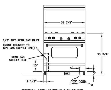
ELECTRICAL CORD LOCATED IN BACK OF UNIT LOCATION OF ELECTRICAL OUTLET MUST NOT BE HIGHER THAN 3" FROM FLOOR IF LOCATED BEHIND THE UNIT OR CAN BE LOCATED IN AN ADJOINING CABINET.
