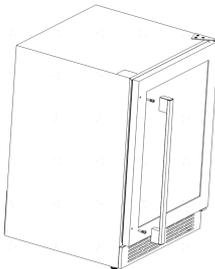
4. Hold the handle and tighten the handle screws with the 1/8" allen wrench.
