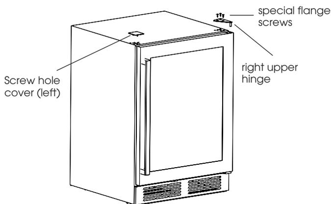
2. Move the door from the hinge by carefully lifting the door straight up.
