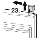
23. Using a screwdriver, push out the plug and transfer it to the opposite side.
