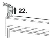
22. Using a screwdriver, push out the hinge and remove it from the door.
