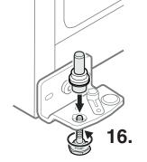
**16.** Tilt appliance slightly backwards, insert pin and attach using the adjustable foot.
