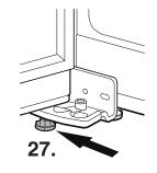
27. Place the appliance in its final position at the place of installation. Extend the adjustable foot at the
