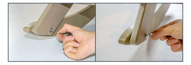
Place the back of the runner on the outside of the back legs. Insert a long bolt into the washer, front leg and runner. Slide on another washer and tighten nut onto bolt.
