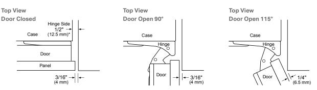
\* Right hand hinge installation shown. When reversing the door, the hinge and handle side clearances also reverse. \*\* Side clearance at front panel
