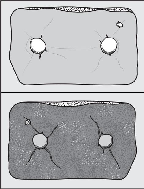
Lint will blow into the heat exchanger through cracks and tears. This will cause a permanent obstruction in the heat exchanger.
