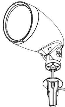
3. Connect the speaker to the stake. The stake has a keyed top that is intended to lock the speaker to the stake. Gently rotate the speaker until you feel it engage with the keyed top. Continue to rotate the speaker. It gradually tightens until it reaches the stop.
