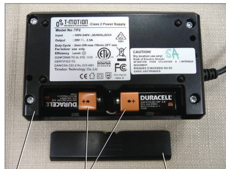
Power Supply (2) 9-Volt Alkaline Batteries Battery Cover
